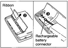
Removing the rechargeable battery:
